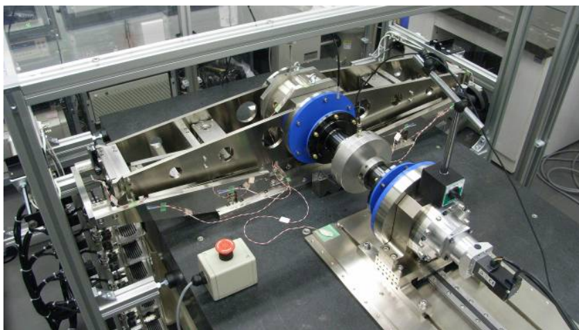
10 N·m deadweight type torque standard machine
