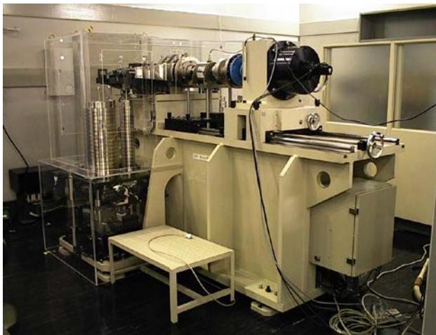
Deadweight type torque standard machines of 1 kN·m (left) and of 20 kN·m (right)
