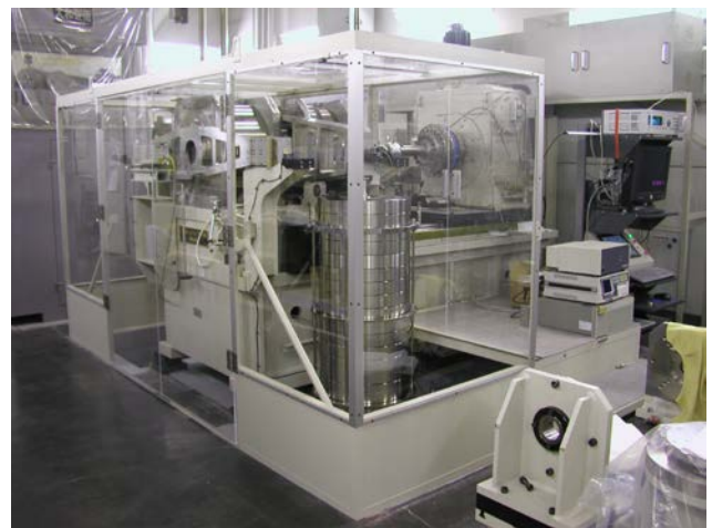
Deadweight type torque standard machines of 1 kN·m (left) and of 20 kN·m (right)
